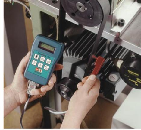
The distance between the drive belt and the measuring probe should be between 3 and 20 mm. See sketch for positioning.
