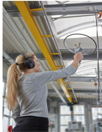
Picture 4: Leakage detection with parabolic dish
