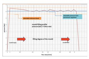
Constant pressure through volumetric flow
