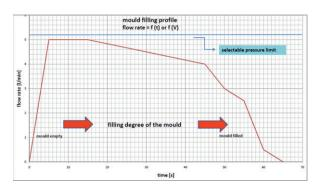
Diaphragm - Volumetric flow profile is defined by the mould filling time.
