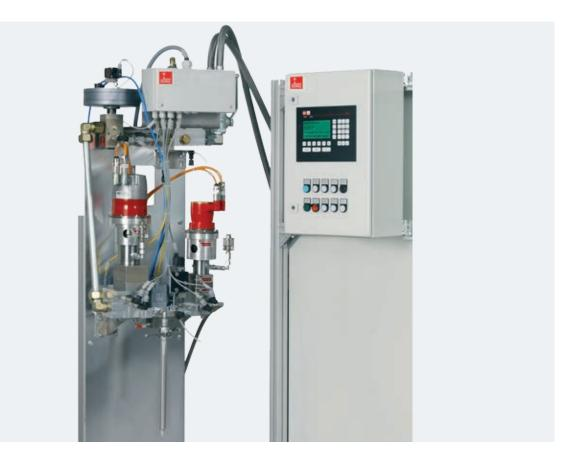
2K-modis is used to handle two component materials. Due to its comptibility and modularity, two modis single component systems can be connecetd by simply using a mixing block onto the outlet of which a plastic mixer is mounted. Just a suitable material supply and metering unit is required.
