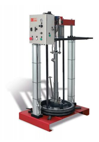
DOPAG drum pumps are chop check pumps. They feed single component media such as greases, oils, adhesives, sealing compounds, polyurethane, silicone etc. with viscosity levels up to 5.0 million mPa s directly and cleanly from original containers.
