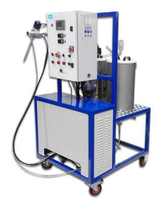
The LiquidFlow 50 is a high-level metering and mixing machine for larger flow production demands. The benefit from this machine is the portable framework with the facility to mount larger material reservoirs and, if requested, a higher flow rate is also achievable. One major advantage of the LiquidFlow 50 is the independent inverter driven motor control for each gear pump, instead of using a lower cost but less efficient gear and toothed belt or chain assembly. This
