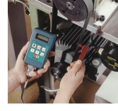
The distance between the drive belt and the measuring probe should be between 3 and 20 mm. See sketch for positioning.
