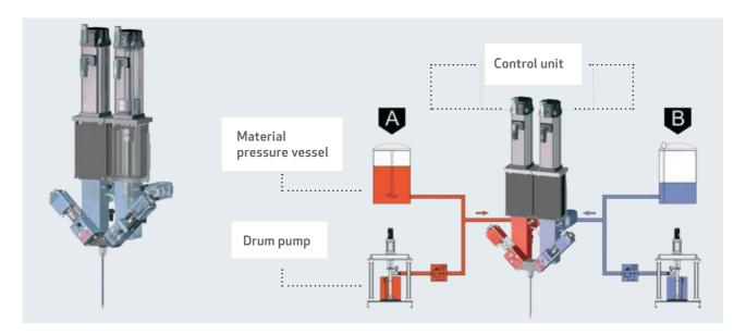
Vectomix is used to handle multi component materials. Due to its compatibility and modularity, two vectodis single component piston metering systems with equal or different sizes are used. They can be connected by simply using a mixing block onto the outlet of which a
